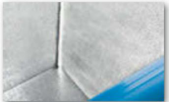
The **powder-coated sheet steel housing** is made from a single sheet of metal and is extremely sturdy and impact-resistant as a result. The 50 mm radiused corners reduce scratches and damage caused by impacts.
