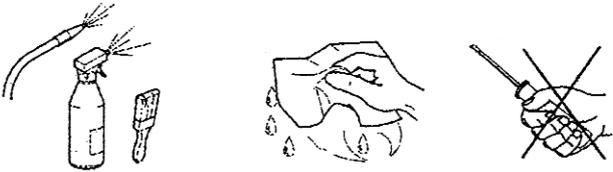
For the cleaning of the unit cabinet use a soft cloth with a mild detergent solution specific for Stainless Steel.
