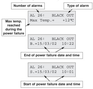
In the case of HIGH/LOW temperature alarms, a pre-alarm time of 60 minutes is counted before they are stored; when this time has elapsed the controller records the alarm in the alarms list and shows the following message on the display:
