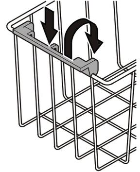
Press the handle downwards, lift and tilt inwards.
